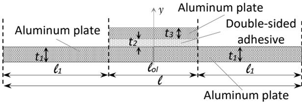
Fig. 4. The configuration of the single strap joint
