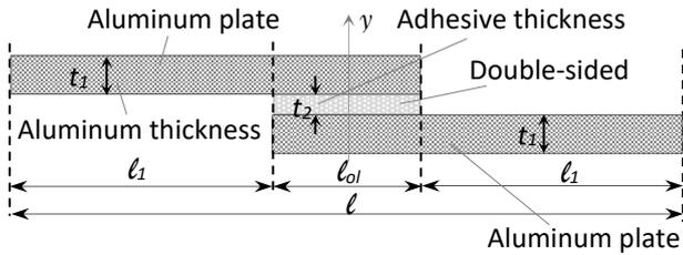
Fig. 3. The configuration of the single-lap joint
