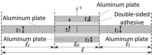
Fig. 5. The configuration of the double strap joint
