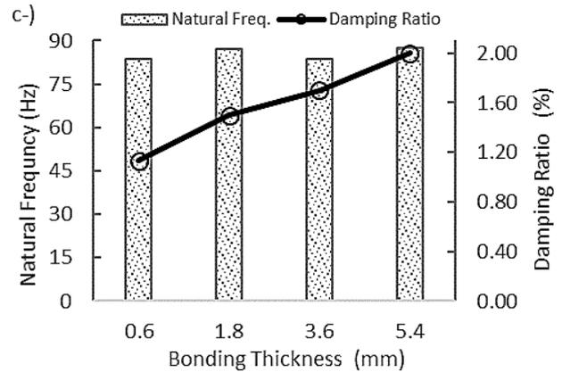
Fig. 6. Variation of natural frequency and damping ratio values of single lap joint; a) overlap length b) aluminium plate thickness, c) adhesive tape thickness
