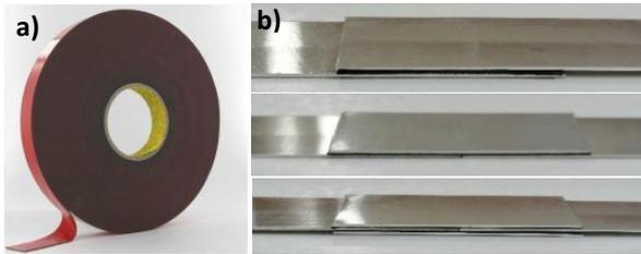
Fig. 1. a) Double-sided tape b) Test specimens of adhesively bonded different joints
