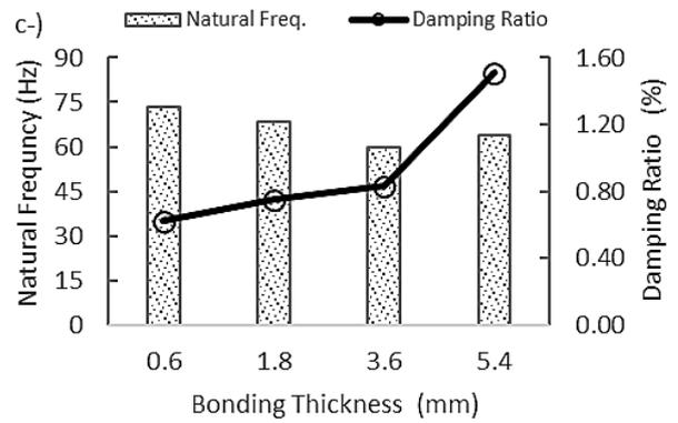
Fig. 7. Variation of natural frequency and damping ratio values of single strap joint; a) overlap length, b) aluminium plate thickness, c) adhesive tape thickness
