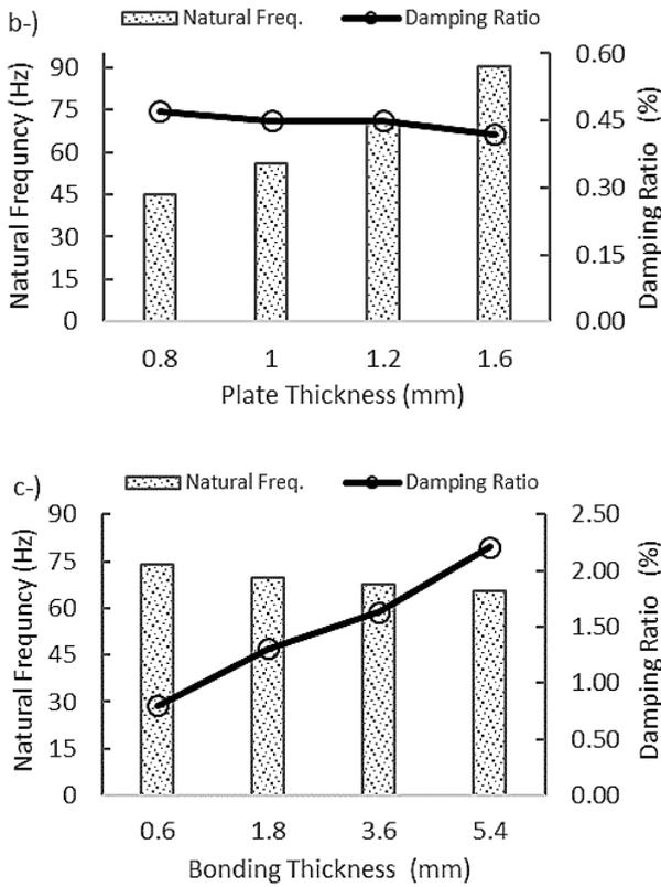
Fig. 8. Variation of natural frequency and damping ratio values of double strap joint with a) overlap length, b) aluminium plate thickness, and c) adhesive tape thickness
