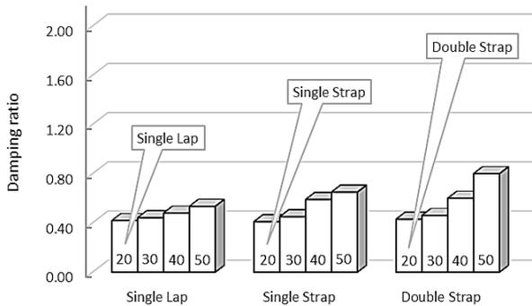
Fig. 9. Comparison of damping ratios of different joint constructions depending on overlap length (20, 30, 40, 50 mm)
