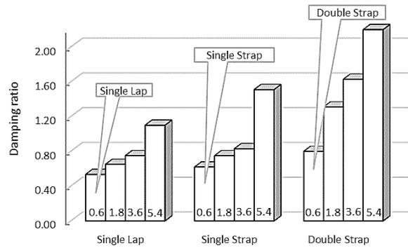
Fig. 10. Comparison of damping ratios of different joint constructions depending on adhesive tape thickness (0.6, 1.8, 3.6, 5.4 mm)
