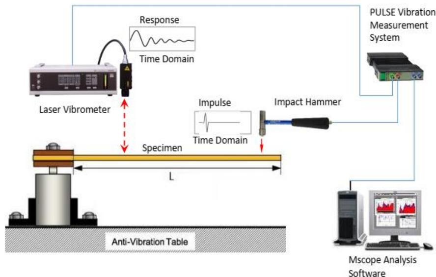
Fig. 2. The schematic of the experimental test set-up
