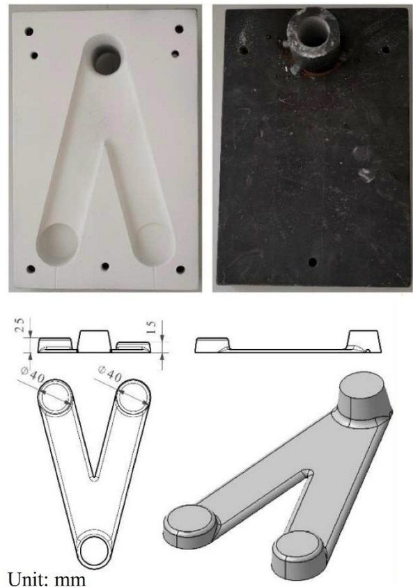
**Fig. 2.** Duck foot mold from different view, and its dimensions.
