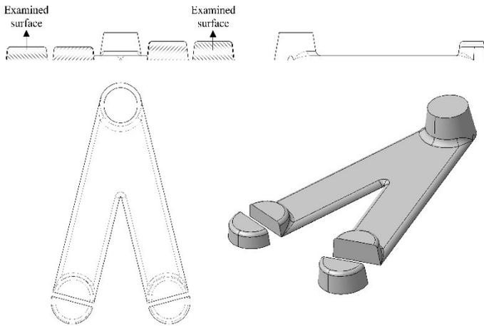
Fig. 3. Schematic views of the cut parts of the cast samples for examination.
