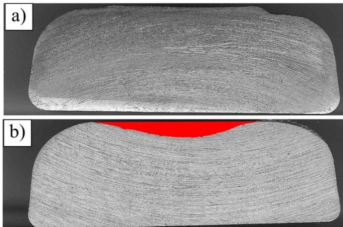
Fig. 4. Shrinkage of duck foot; a) without cleaning, b) after cleaning.
