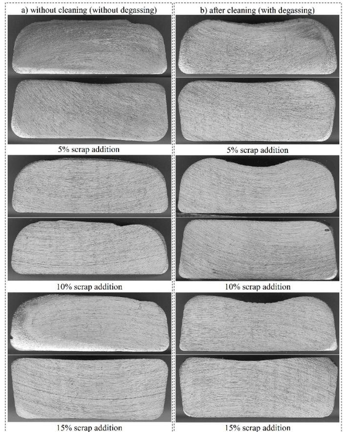
Fig. 6. Display of shrinkage amount of duck foot small and large pieces a) without cleaning, b) after cleaning.
