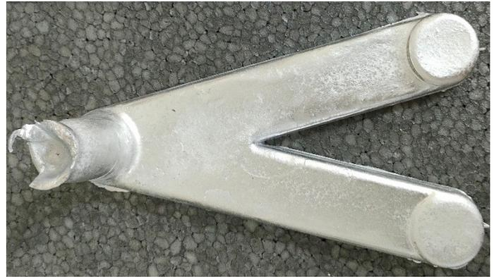
Fig. 5. Duck foot mold casting sample.
