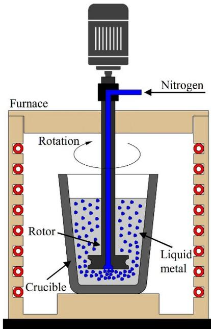
**Fig. 1.** Schematic view of the liquid metal cleaning process with rotary degassing.
