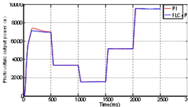
Fig. 6. (b) Output power under partial shadow
