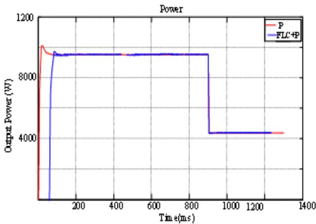
Fig. 5. Output power under insolation/irradiance levels from 9560 to 4560 W/m<sup>2</sup>
