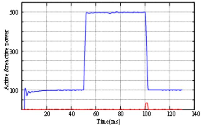
Fig. 9. (f) Active and reactive power during acceptance test
