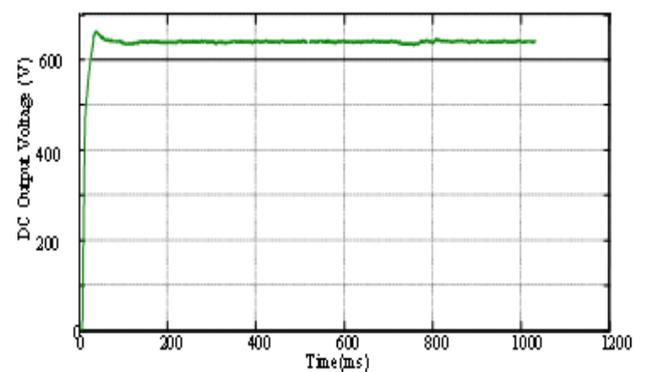
Fig. 9. (a) DC bus voltage at night
