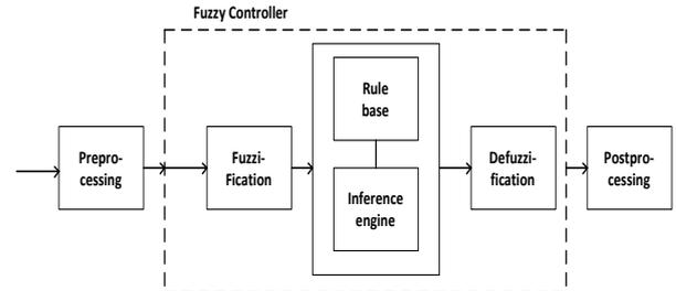
Fig. 2. Fuzzy controller structure
