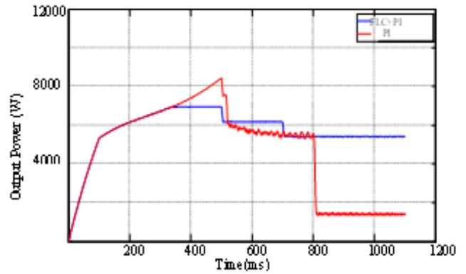
Fig.7. Output power under partial shadow when the battery bank is disconnected
