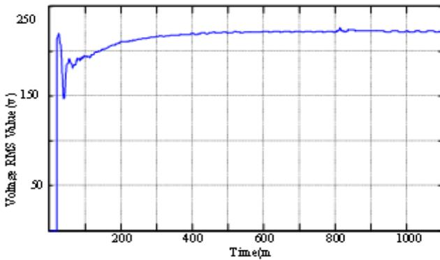
Fig. 9. (c) Inverter  $V_{rms}$  value for one phase
