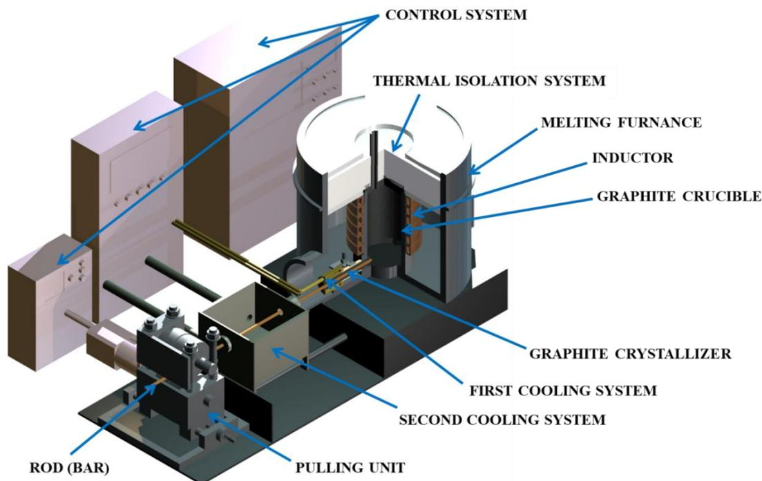
Fig. 1. Laboratory line for continuous horizontal casting non-ferrous metals and alloys
