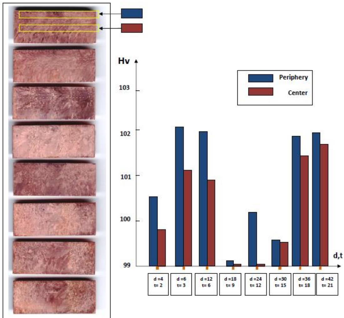
Fig. 7. Vickers hardness variation in peripheral and central zone of the Cu-Mg alloy rod during the increasing the pull distance and the pause time.
