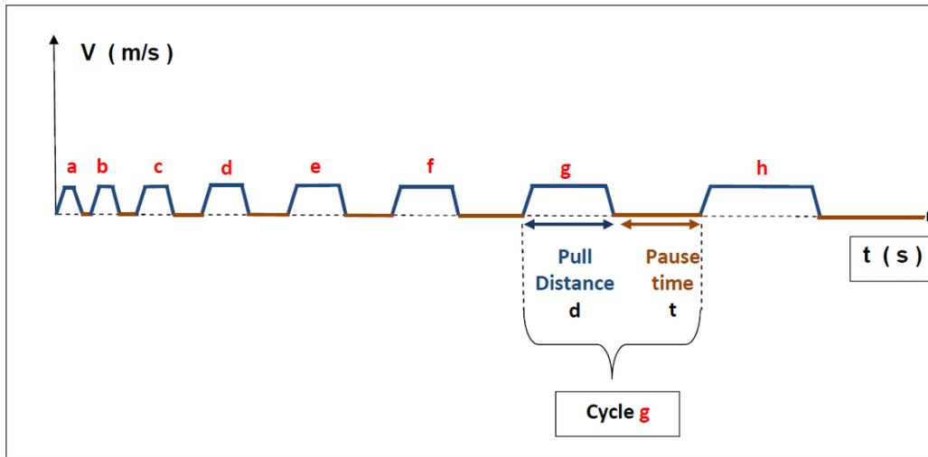
Fig.2. Withdrawn cycles( Casting speed  $V$  vs time  $t$  ) during the continuous horizontal casting process of Cu-Mg alloy : ( a ) :  $d= 4\text{mm}$   $t = 2\text{s}$ , ( b ) :  $d= 6\text{mm}$   $t = 3\text{s}$ , ( c ) :  $d= 12\text{mm}$   $t = 6\text{s}$ , ( d ) :  $d= 18\text{mm}$   $t = 9\text{s}$ , ( e ) :  $d= 24\text{mm}$   $t = 12\text{s}$ , ( f ) :  $d= 30\text{mm}$   $t = 15\text{s}$ , ( g ) :  $d= 36\text{mm}$   $t = 18\text{s}$ , and ( h ) :  $d= 42\text{mm}$   $t = 21\text{s}$ .
