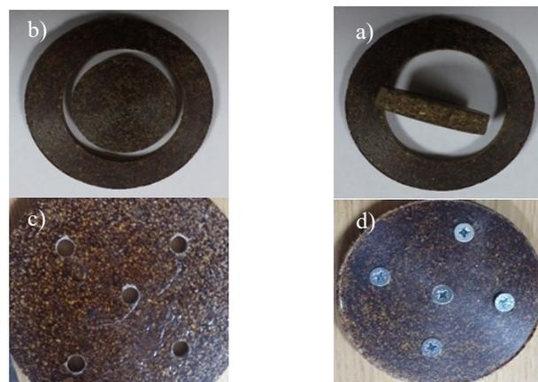
Fig. 1. Machinability properties of produced composite material a-b) punching process c) drilling process d) screwed joint process
