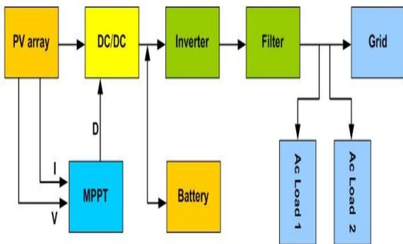
Fig. 1. Integrated PV-Battery- Inverter-Smart grid system
