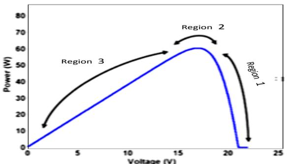
Fig. 2. (a) The algorithm of perturb and observe (P&O), (b) Proposed of perturb and observer, (c) PV cell (Power/Voltage) curve operating regions
