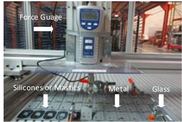
Fig. 3. Glass strength/tensile test mechanism
