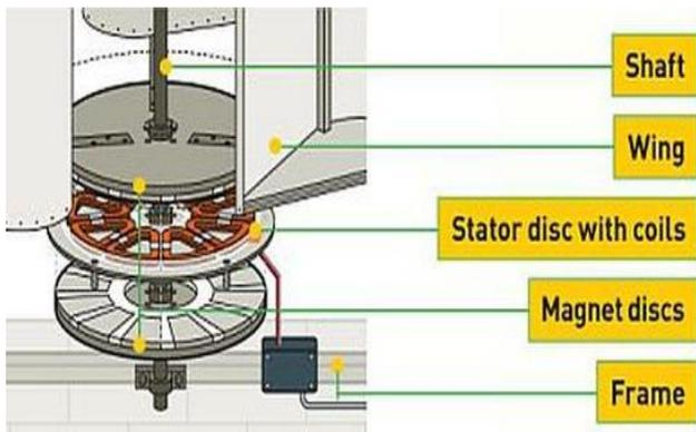
Fig. 5. The constructed vertical axis wind turbine and the components [21].
