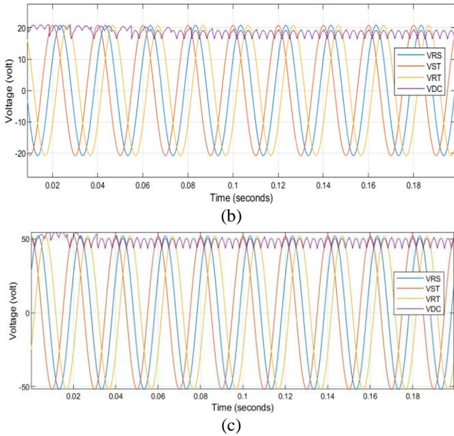
Fig. 9. Three input voltage for (a) 5V, (b) 12 V, (c) 30 V maximum phase and rectifier output voltages.
