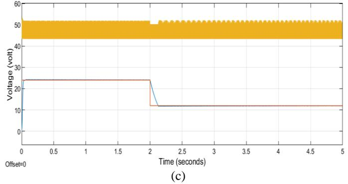
Fig. 10. The simulation results for rectified input voltages (a) 8V, (b) 19V, (c) 50V and for different references (12V, 24V).
