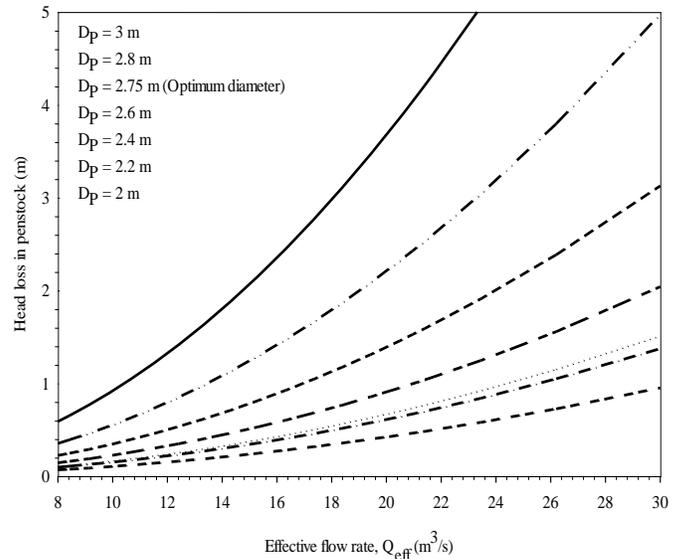
Fig. 16. Head losses for different effective flow rates and penstock diameters.
