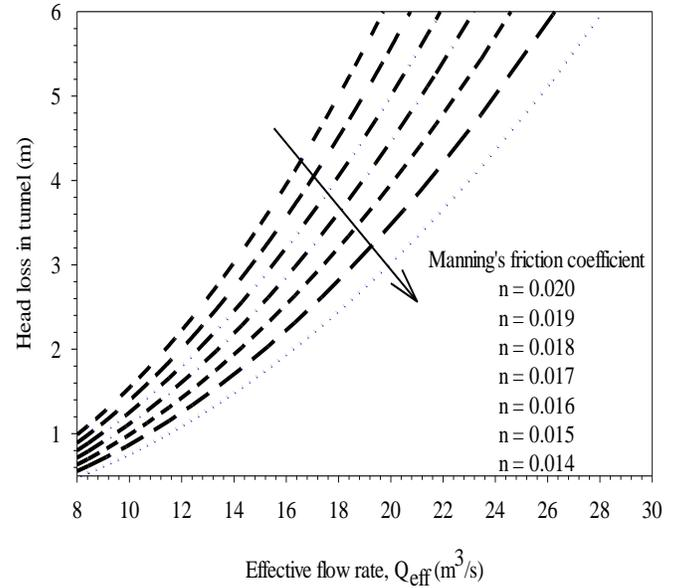
Fig. 12. Head losses depend on Manning's friction coefficient and effective flow rate for optimum tunnel diameter.
