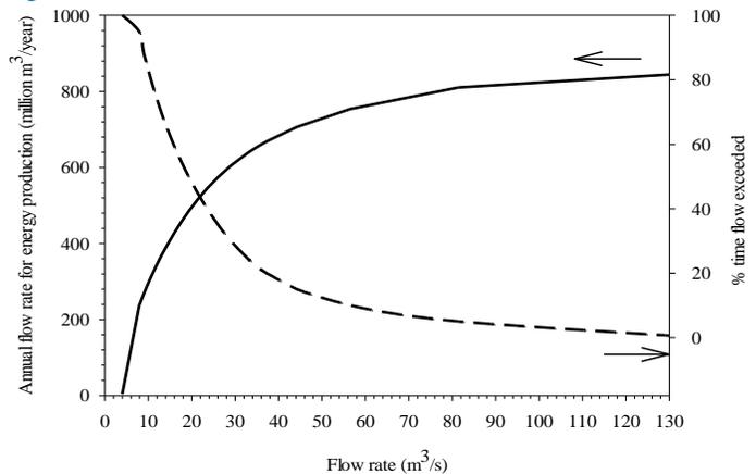
Fig. 4. Annual flow rates for energy production and % time flow exceeded for different flow rates.
