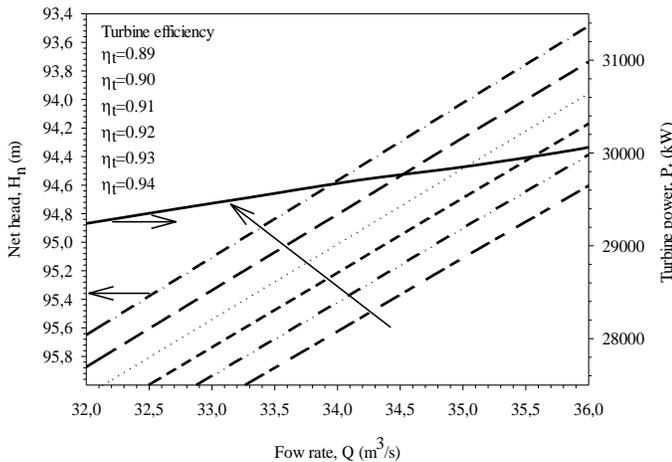
Fig. 18. Variation of turbine power for different flow rates, net head and turbine efficiency.
