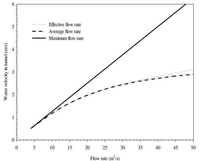
Fig. 13. Variations of water velocity in air-shared transmission tunnel for optimum tunnel diameter.
