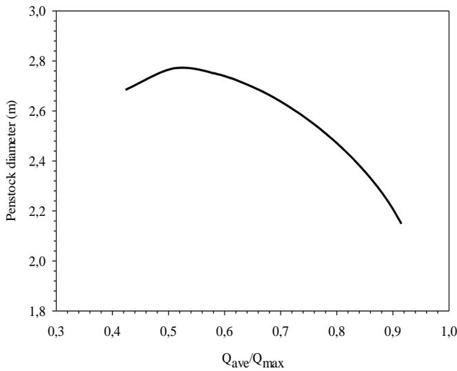
Fig. 15. Variation of penstock diameter with  $Q_{ave}/Q_{max}$ .
