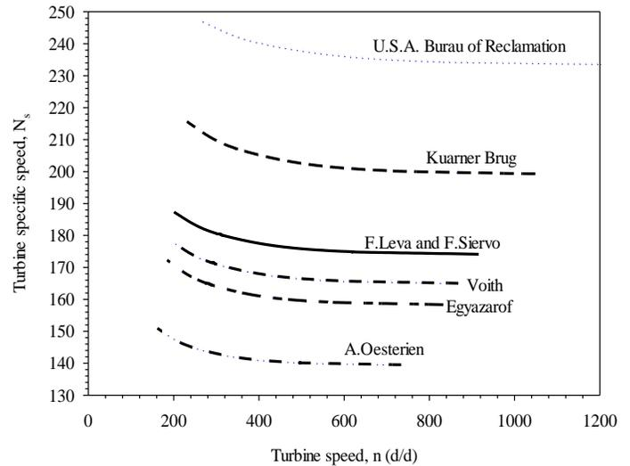
Fig. 20. Variation of turbine speeds depending on the turbine specific speed for different turbine manufacturers.
