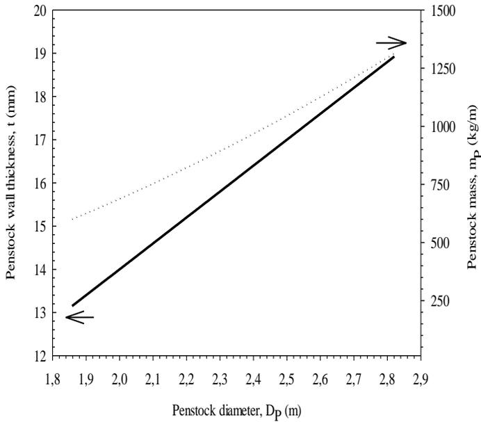
Fig. 14. Variations of penstock wall thickness and penstock mass depend on the penstock diameter.
