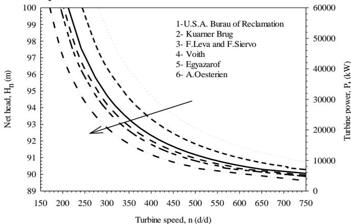
Fig. 19. Different turbine manufacturers give turbine speeds to obtain total turbine power depending on the net head.
