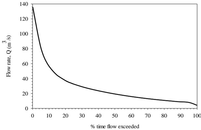
Fig. 2. Flow duration curve.
