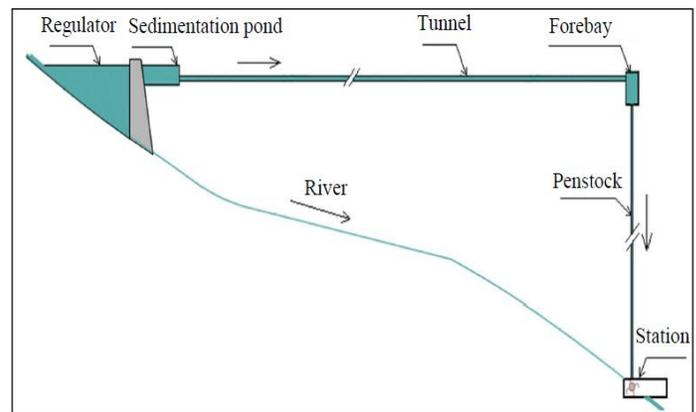
Fig. 1. A general view of a regulator-type hydropower plant.
