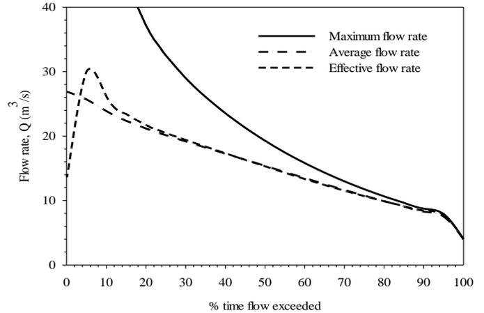
Fig. 3. Maximum, effective and average flow rates for various flow rates and % time flow exceeded.
