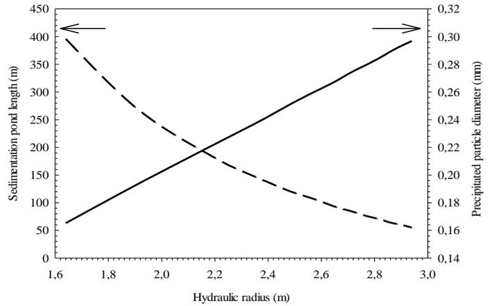
Fig. 5. Sedimentation pond length and particle diameter depend on the hydraulic radius for project flow rate.
