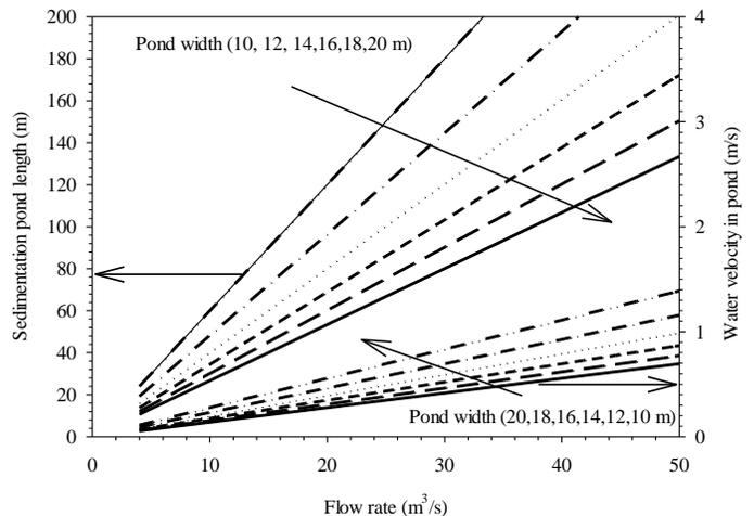
Fig. 6. Sedimentation pond length and water velocity in pond depending on the flow rate for different sedimentation pond widths.
