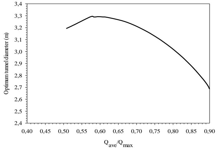
**Fig. 8.** Optimum tunnel diameter for different values of  $Q_{ave}/Q_{max}$ .
