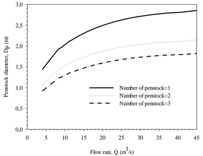
Fig. 17. Variation of penstock diameter depending on flow rate and the number of the penstock.
