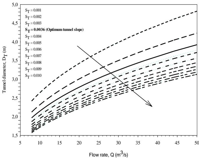
**Fig. 7.** Variation of tunnel diameter depending on tunnel slope and flow rate.
