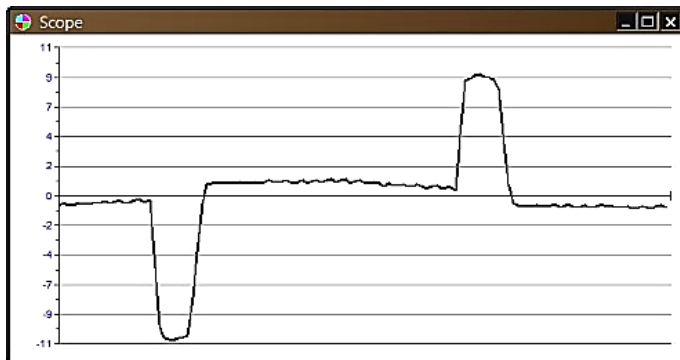
Fig. 7. The current waveform of B (75 W) LED lamp.
