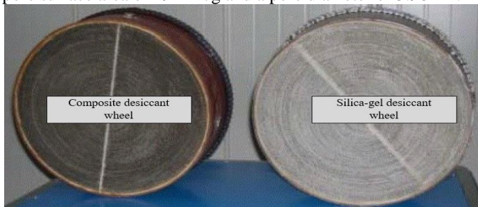
Fig. 7. Pictures of the developed composite and SG-based RDW [24].
