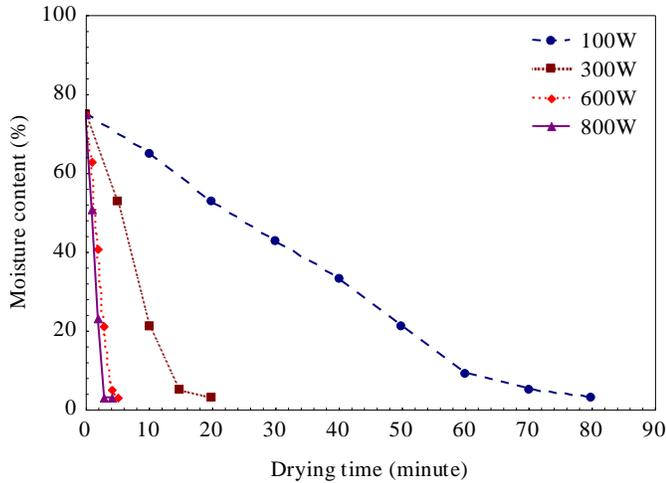
Fig. 5. The variation of moisture content with time.
