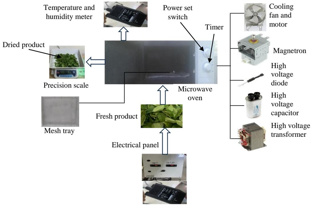
Fig. 2. Flow chart of the microwave drying system.
