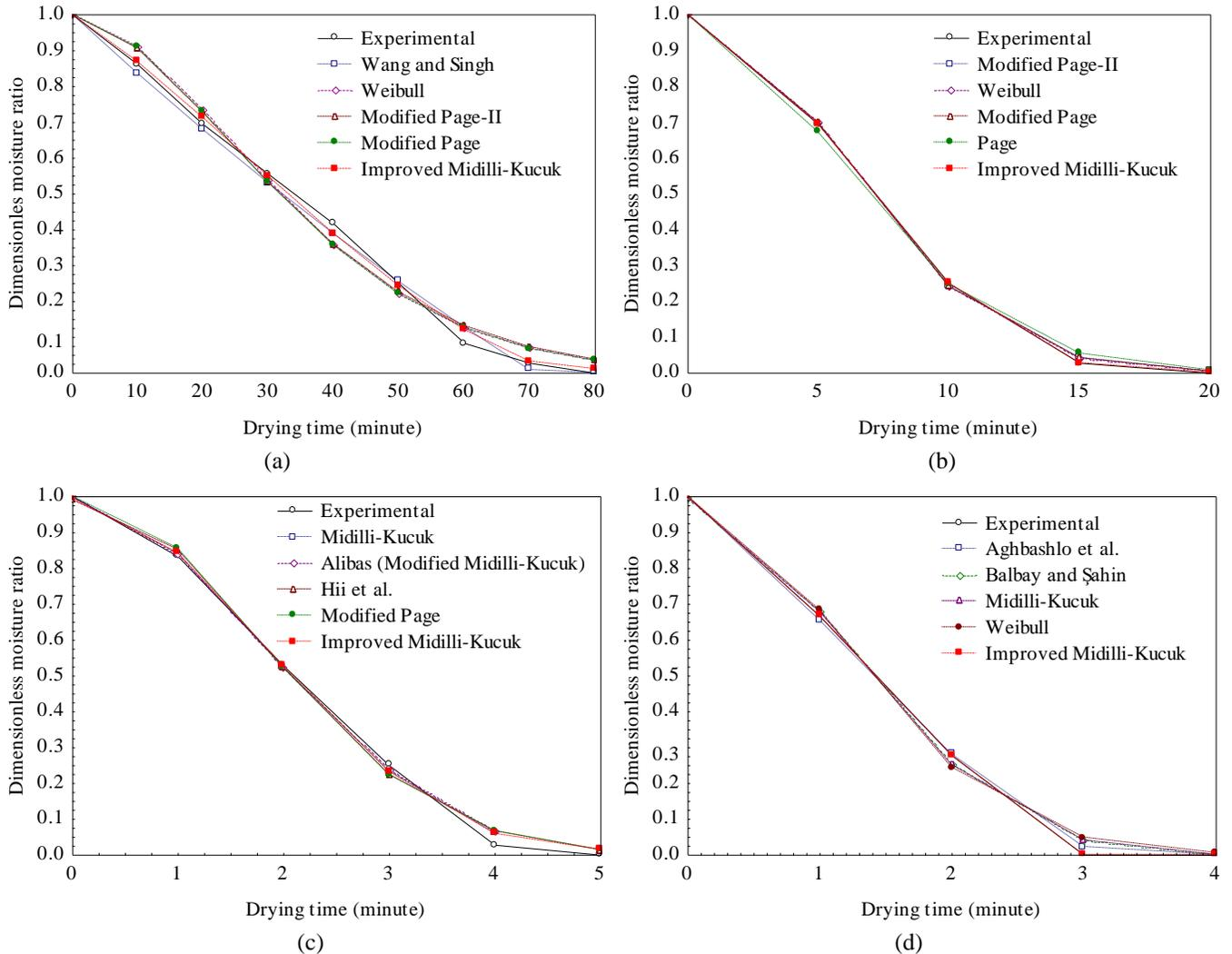
Fig. 3. Variation of MR with time, (a) 100 W, (b) 300 W, (c) 600 W, and (d) 800 W.
