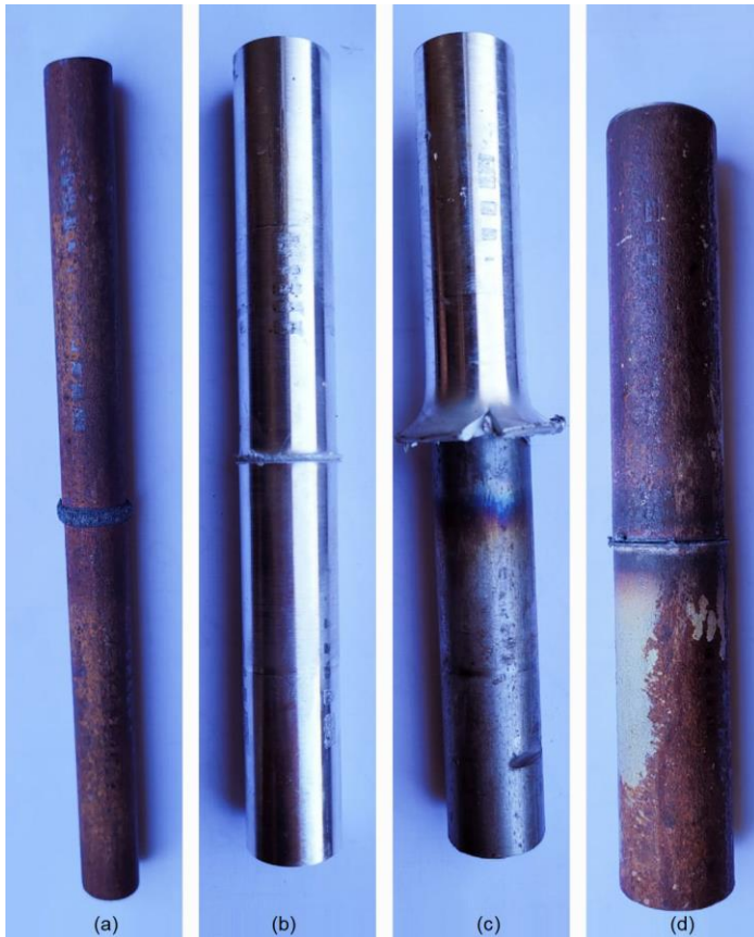
Fig. 12. Welded samples; (a) steel to steel, (b) Al to Al, (c) steel to Al, (d) steel pipes.
