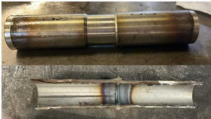
Fig. 13. Cut section of the welded steel pipes.
