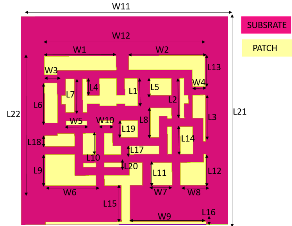
Fig. 3. Design of the proposed patch antenna.
