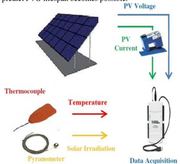
Fig. 2 (a). Real-time data acquisition for each PV plant
