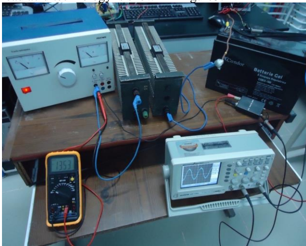
Fig.5.Used lead acid battery and test setup
