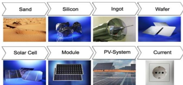
Fig. 4. The main manufacturing steps of solar cells.
