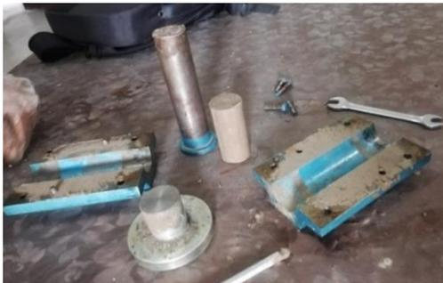
Figure 2-13 Unconfined Test Mold
