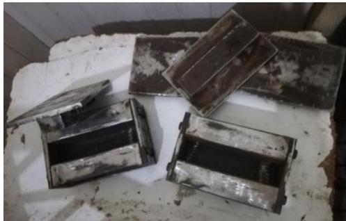
Figure 2-5 Flexural test mold
