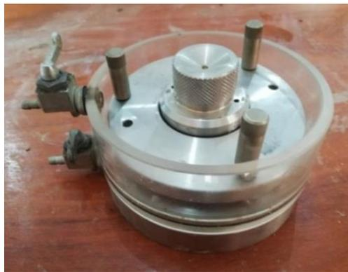
Figure 2-16 Consolidometer
