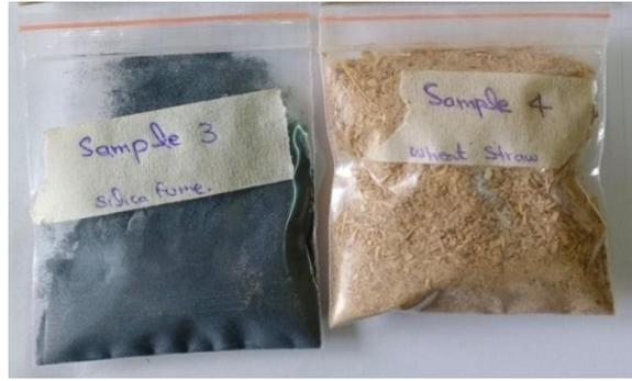
Figure 2-1 Micro Silica Fume and Powder Wheat Straw
