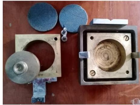
Figure 2-12 Direct Shear Testing Box
