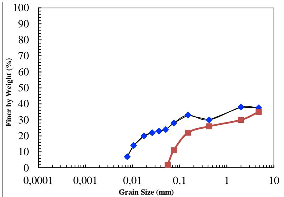
Figure 2-4 Grain size Distribution Chart of Local Soil
