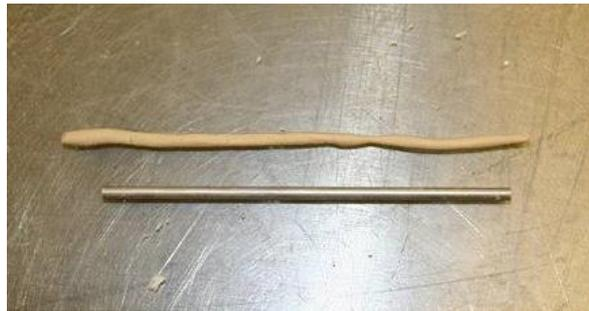
Figure 2-6 Soil Thread made to find Plastic Limit of soil specimens
