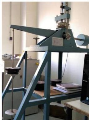
Figure 2-6 Oedometer Frame
