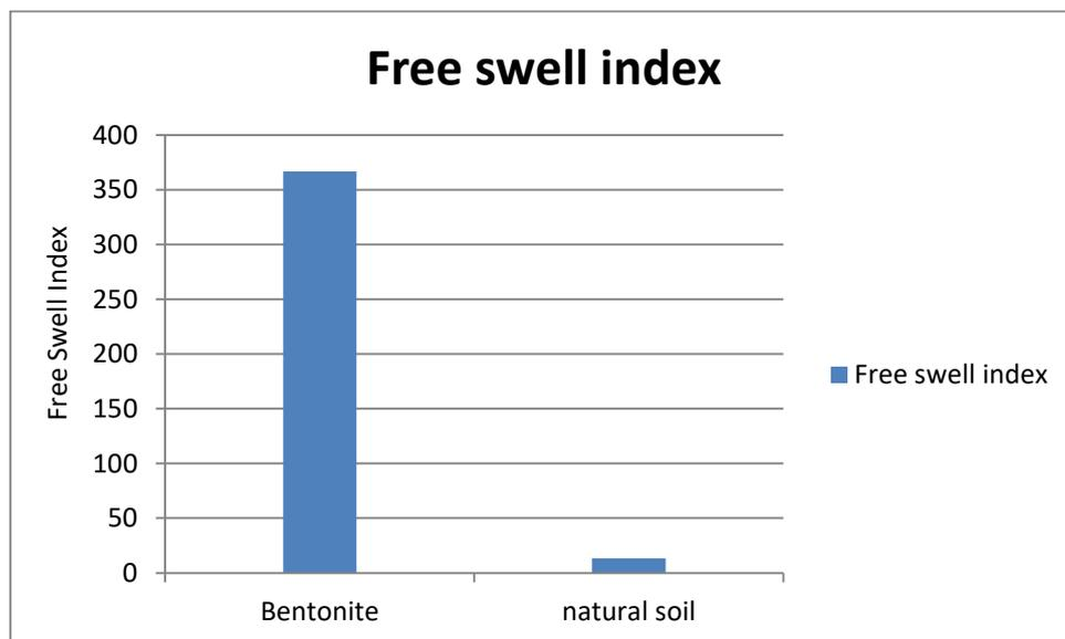
Figure 2-3 Free Swell Index Test Results for Bentonite and & Local Soil
