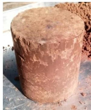
Figure 2-3 Standard Compaction Test Specimen
