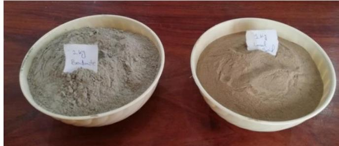
Figure 2-2 Bentonite & Local Soil
