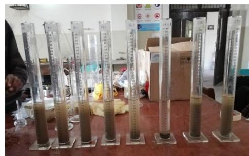
Figure 2-10 Specimens under Observation in Free Swell Index Test
