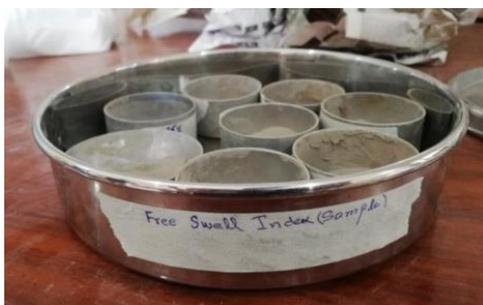
Figure 2-4 Specimen for Free Swell Index Test with Different Proportions of Binary Additive
