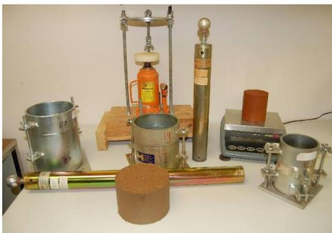
Figure 2-2 Standard Compaction Test Apparatus
