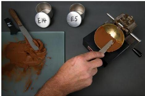
Figure 2-1 Applying Soil in Brass Cup of Casagrande Apparatus
